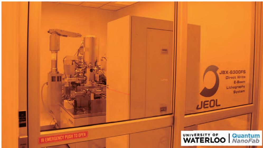
JEOL JBX-6300FS Electron Beam Lithography system, as installed at University of Waterloo Quantum NanoFab. Photo credit: University of Waterloo
