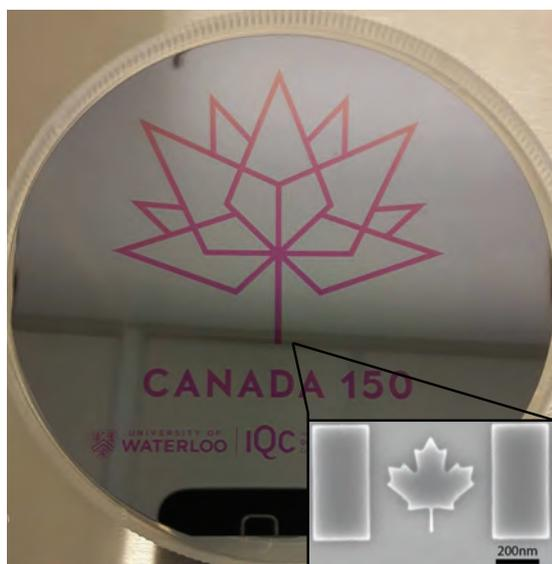
Photograph of completed wafer with electron micrograph of nanoscale Canadian flag inset. Photo credit: University of Waterloo
