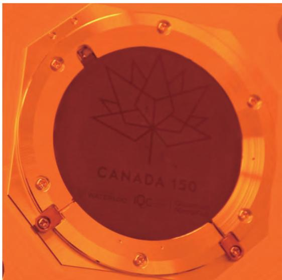
Photograph of HSQ coated 100 mm wafer with Canada150 logo. Wafer is mounted in cassette prior to exposure in JBX-6300FS. Photo credit: University of Waterloo
