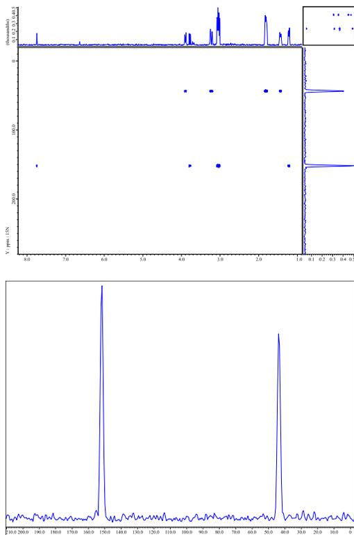
**Figure 7. (Top) H-N gHMBCAD of brucine (50 mg, chloroform-d). Sampling: 50%. Total acquisition time approximately 20 minutes. (Bottom) Projection of the Y-dimension as a 1D  $^{15}\text{N}$  spectrum.**
