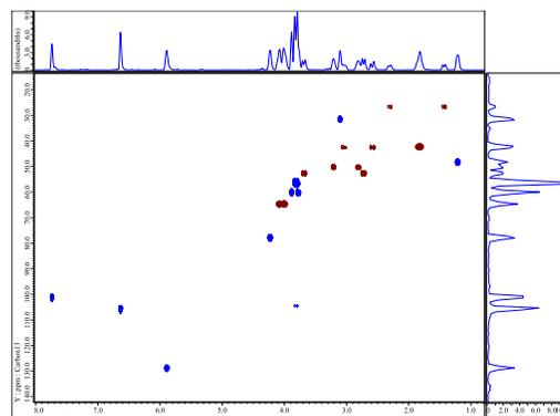
**Figure 8. CRISIS-HSQCAD of brucine (50 mg, chloroform-d). Sampling: 25%. Total acquisition time approximately 5 minutes.**
