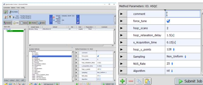
**Figure 9. A sample automation method. Note the simple toggles for sampling type, number of Y points, and sampling rate. These can be customized as the user desires.**
