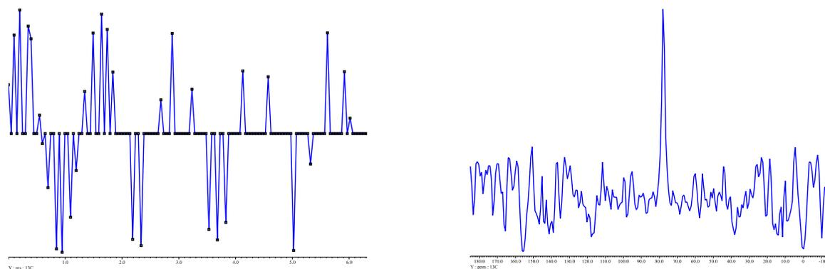
Figure 2. (Left) A time-domain Y slice of an HSQC collected with 25% sampling. Missing increments are replaced with zeroes. (Right) Result of a Fourier Transform of the data.
