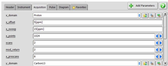
Figure 10. The acquisition tab of an HSQC experiment.
