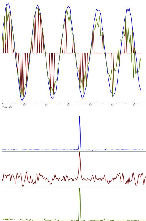
Figure 4. (Top) Overlay of the time-domain Y slice of conventionally sampled data (blue), 25% sampled data with zero-filling of missing points (red) and the reconstruction of the 25% sampled data (green). (Bottom) Result of the Fourier Transform of the data.
