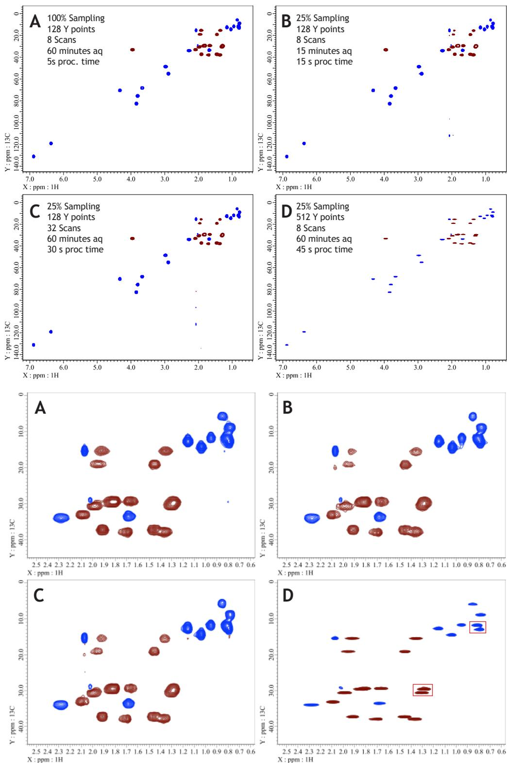
Figure 6. (Top) C<sup>2</sup>HSQC spectra of lasalocid at 400 MHz (Bottom) Expansion of the aliphatic region. Note the peaks that are resolved with 512 Y points (Spectrum D)
