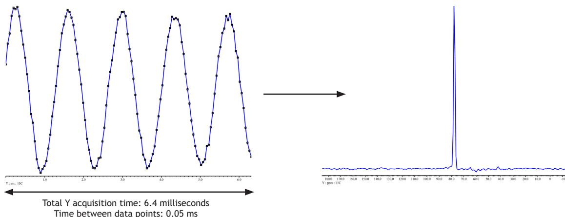
Figure 1. (Left) A time-domain Y slice of an HSQC. (Right) Result of the Fourier Transform. Black squares correspond to the actual data points.
