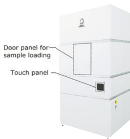
Opening a door in the center part of the microscope cover, sample loading position appears. After placing the specimen transfer cup at the sample loading position, specimen magazine is automatically loaded into CRYO SPECPORTER™ when the button on the touch panel is turned on. Inside the cover there is stored an automated liquid nitrogen filling system besides the main column of the microscope. The inner surface of the cover is soundproofed.
