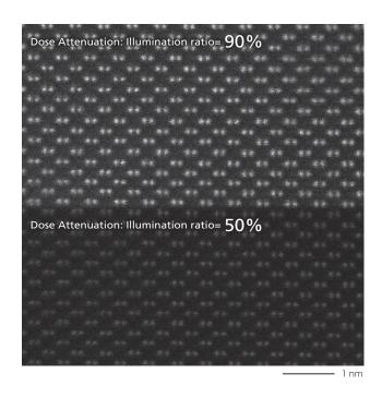
Dose attenuation by pulsed illumination with Frequency of 500 kHz (2  $\mu$ s) in a high resolution STEM at 300 kV using Si [110] in the condition of pixel dwell time with 19  $\mu$ s/pixel (1024  $\times$  1024 pixels), by changing duration ratio from 90% to 50% during acquisition of one STEM image in 20 s.
